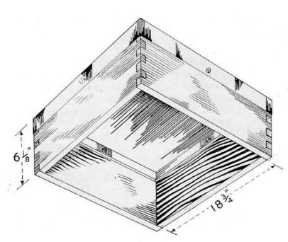
tions, then fit the top boards, nailing them through onto the side boards along all four sides. Next fit the four strips to provide the head space, then cover with waterproof cover (metal or tarred felt) before completing the ventilation holes.
