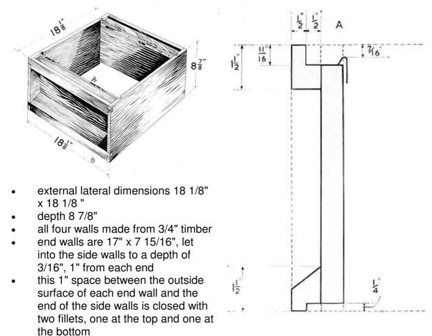
• top fillet rebated on the inside 11/16" deep from the top edge, leaving a shoulder 1/2" wide - this rebate forms part of the recess which encloses the ends of the frame lugs
